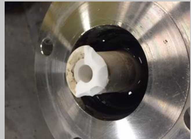
Hydro cyclone ceramic piece broke
